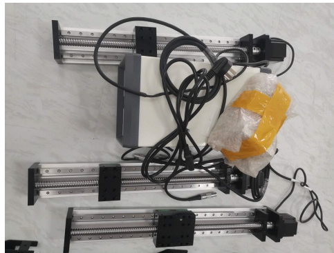
Figure 5: A typical traverse system consists of 1 controller, 3 modules, cables, and connectors.
