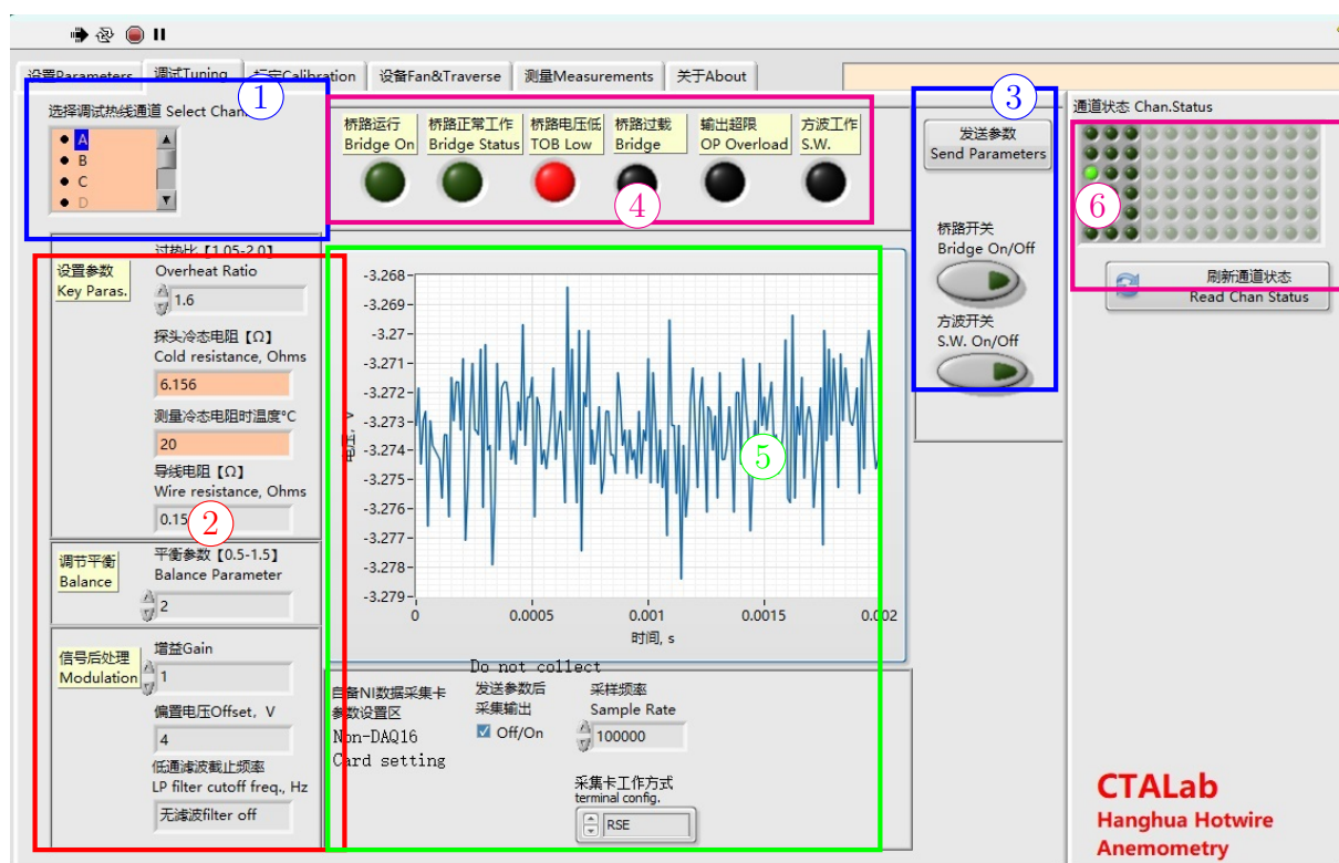
Figure 15: The Tuning tab is divided into different functional areas: ① Channel selection, ② Setting channel operating parameters, ③ Sending parameters, switching the bridge on and off, and square wave testing, ④ Current channel status indicator, ⑤ Current channel voltage output waveform, and ⑥ Status indicators for all channels.
